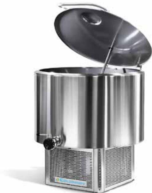
The FREECOLD milk tank cools a 150 liters milking in 2 hours down to a temperature of 4 °C with an ambient temperature of 35 °C.
